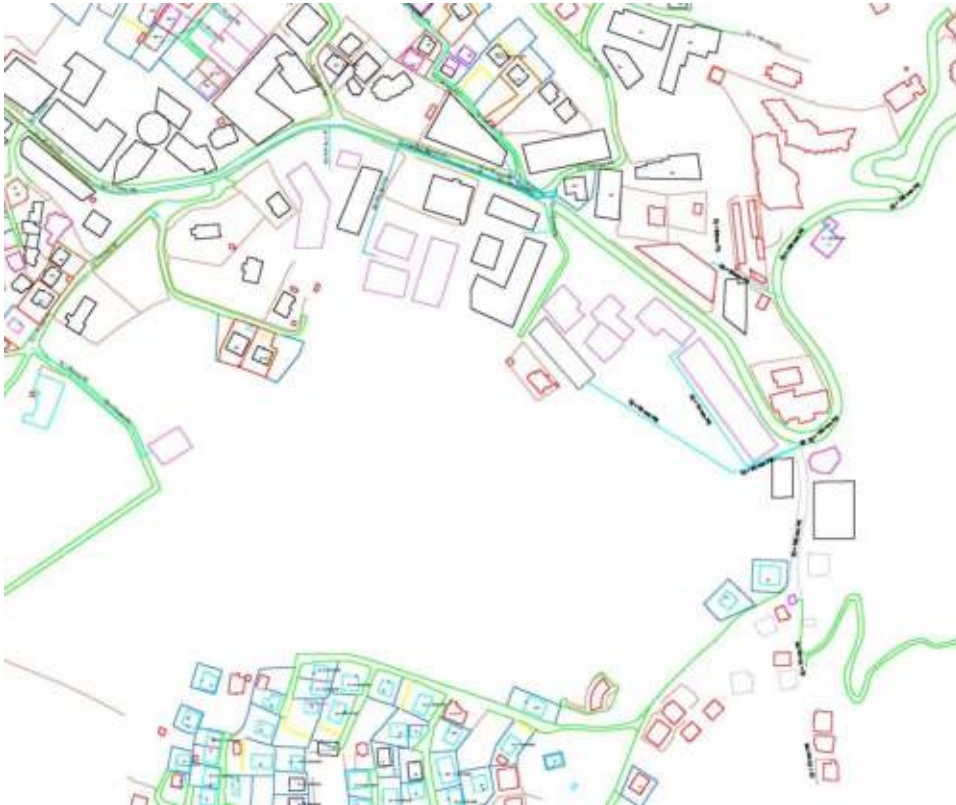
Map 37 – Situation of sewerage network in the site
